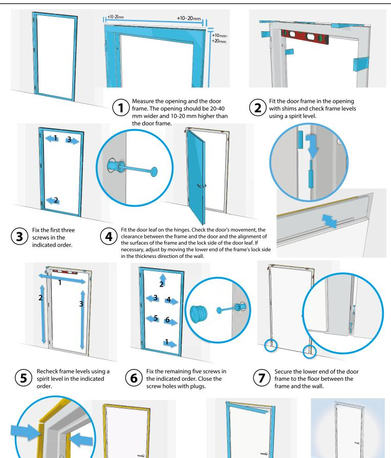
Insulate the gaps between the frame and the wall with stone wool and remove the shims. Insulate fire doors with Paroc Extra stone wool. For metal fire doors EI2 30 and EI2 60 in stone walls, Wurth Fire Protection and Soudafoam Gun FR HY polyurethane foams can also be used.
