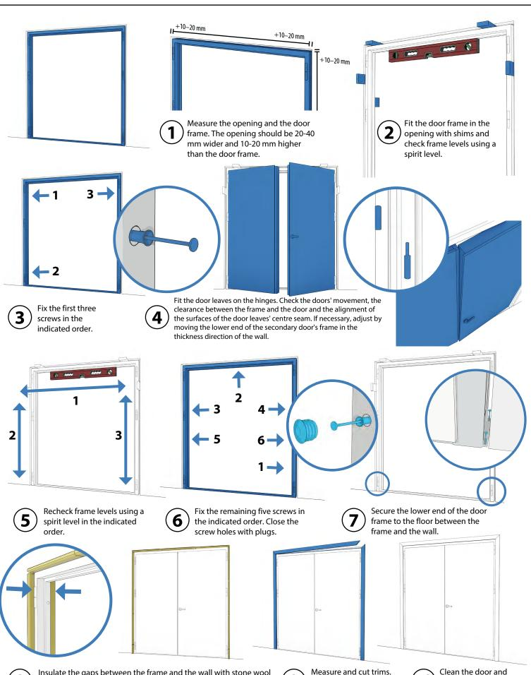
Insulate the gaps between the frame and the wall with stone wool and remove the shims. Insulate fire doors with Paroc Extra stone wool. For metal fire doors EI2 30 and EI2 60 in stone walls, Wurth Fire Protection and Soudafoam Gun FR HY polyurethane foams can also be used.
